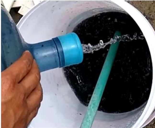
**Add sufficient clean water (10-20 times) to dilute sulfuric acid to prepare filtering.** Rinse several times before final filtering. Strong sulfuric acid will damage the filter paper if not diluted properly
