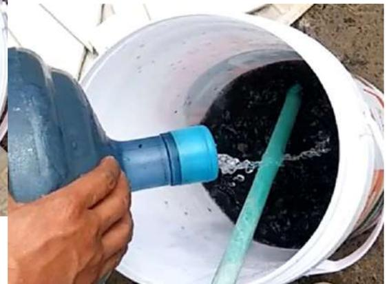
Slowly add diluted HCl or H<sub>2</sub>SO<sub>4</sub> solution prepared into the pail to dissolve loaded zinc strips
